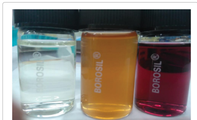
Figure 1: Colour Change during phytochemical reduction of chloroauric acid to ruby red colour.
