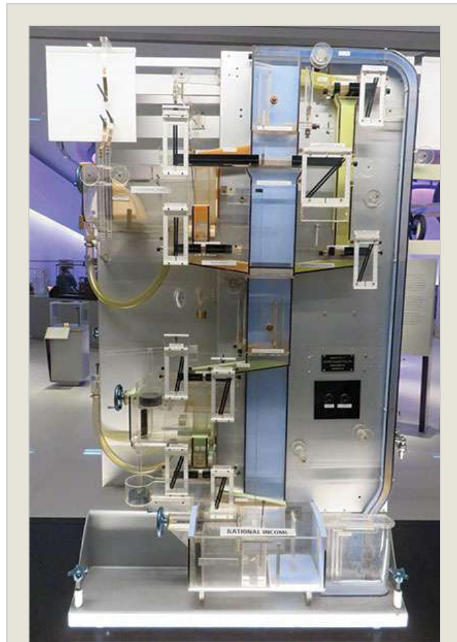
Figure 2.3 'Moniac' uses water to compute the way money flows through the UK economy.
