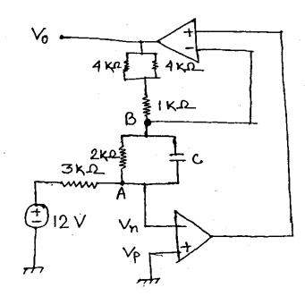
7. What is schmitt trigger? Explain its operation sketch its transfer characteristics and indicate the hysteresis.
